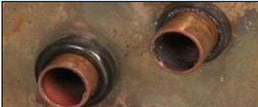
Annealed Fins – Low Water Flow
