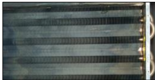
Sooted – Improper Fuel and Air Mixture.
