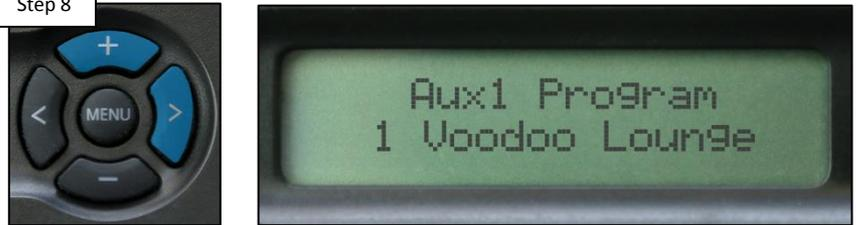
Press the (>) to navigate through the Setting Menu, press the (+) to enter each relay and fine tune brightness, colors, shows..etc.
