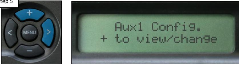
Once complete, navigate to each relay you wish to control the lights through by pressing the (>), press (+) to enter each relay.
