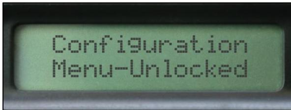
Press the Menu button until "Config. Menu – Locked" appears, then press and hold the (<) & (>) until "Unlocked".
