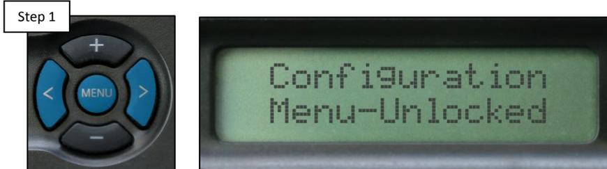
Press the Menu button until "Config. Menu – Locked" appears, then press and hold the (<) & (>) until "Unlocked".
