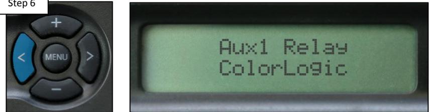
Press the (>) to locate the relay type and change it to "ColorLogic" by pressing the (+), then press (>) to assign lights.
