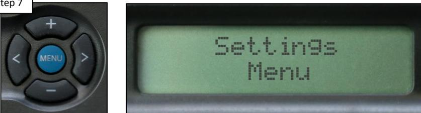
Once all the desired relays are set to "ColorLogic", press the "Menu" button until the "Settings Menu" appears.
