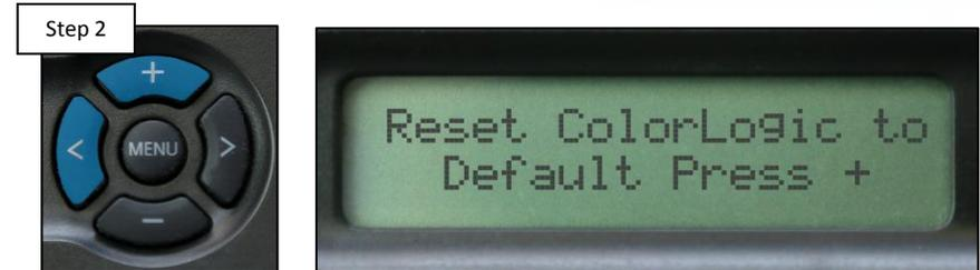
Press the (<) until "Reset ColorLogic to Default." appears on the screen, then press the plus (+) to enter.
