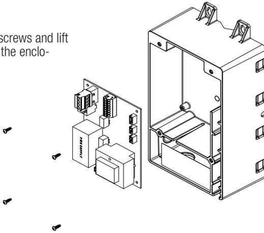
4. Unfasten the VS Omni Hub enclosure from the mounting surface and remove.
