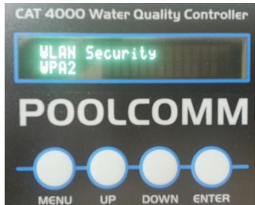
6) Select the security setting used by your router. Security setting types are shown below and can be found on your router or by contacting your internet service provider.\*
