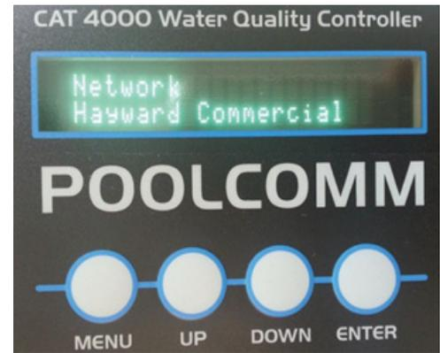
4) Scroll down to find your wireless network. Press ENTER to select. If display shows “None”, then please allow an additional 5 minutes for unit to try to find networks.
