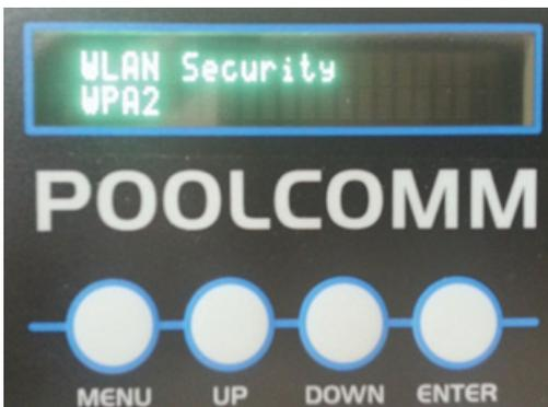
7) Using the UP and DOWN buttons, input the password then press ENTER. Allow at least 5 minutes for unit to establish network connection, depending on your wireless network speed. Test the connection by pressing the “Transmit” button.
