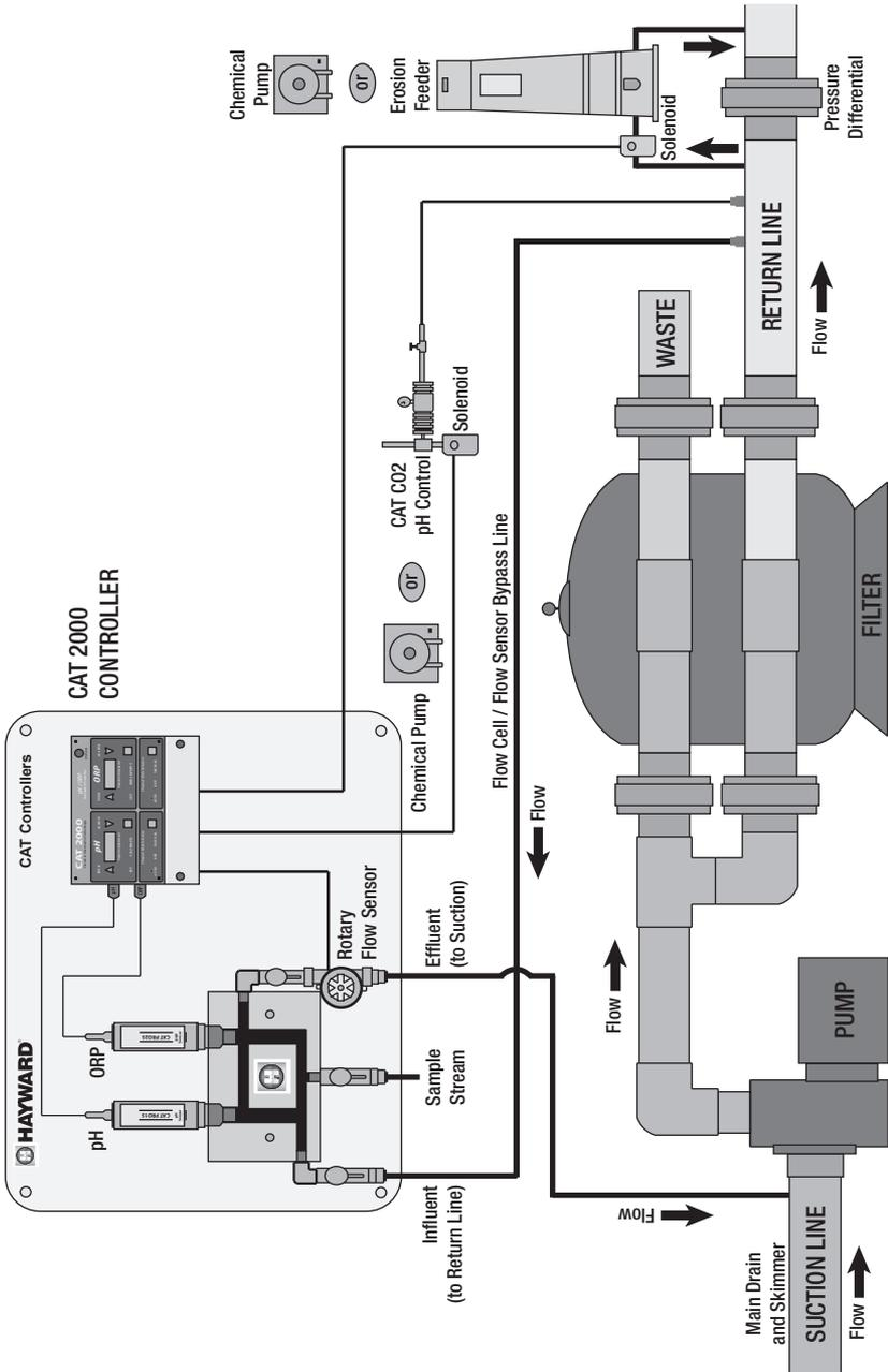
ALL CHEMICALS MUST BE INJECTED DOWN STREAM FROM HEATER AND FLOW CELL
