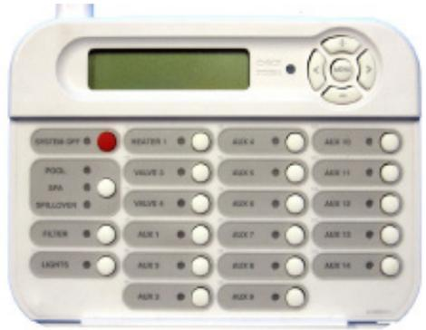
Shown below is a labeled remote control to a Pro Logic PS pool control. Note that labels have been placed over the generic names to describe the equipment being controlled. In this case, the Pool Filter, Gas Heater, Spa Filter and Water Feature are all turned on.
